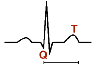
The QT interval is the time between the Q and the T wave in an electrocardiogram (ECG).
